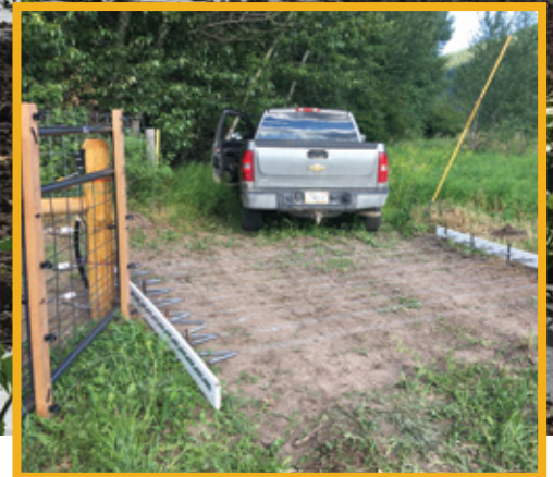
This is a drive-over gate, one of four experimental gates going into the melon field, designed to allow vehicle but not bear entry.
